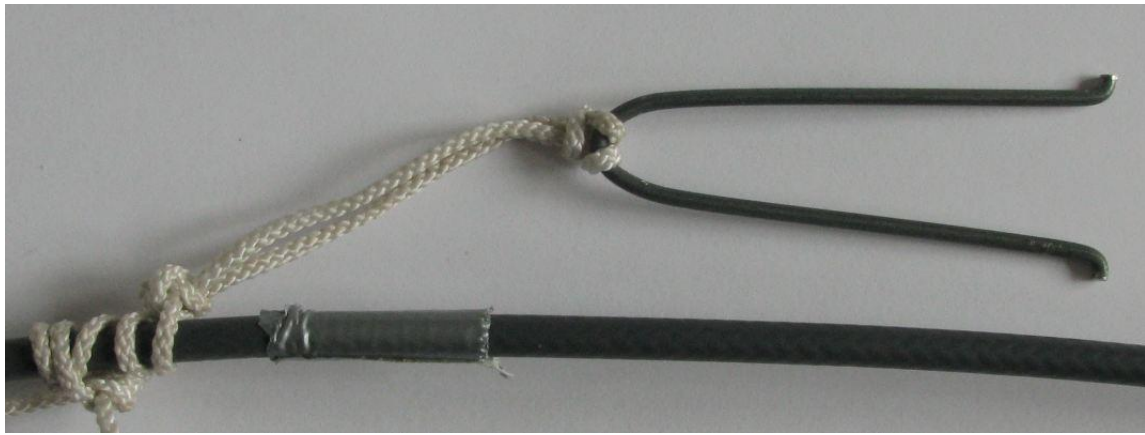
Figure 4.5, Strain relief spring connected to Belden H155 cable.
