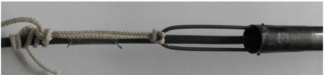
Figure 4.6, Strain relief in action
