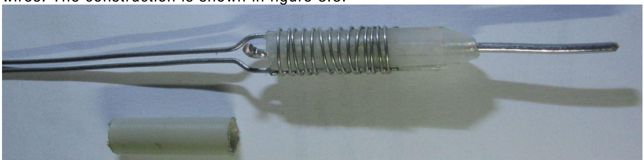
Figure 3.3, Ground wire construction and coil former
