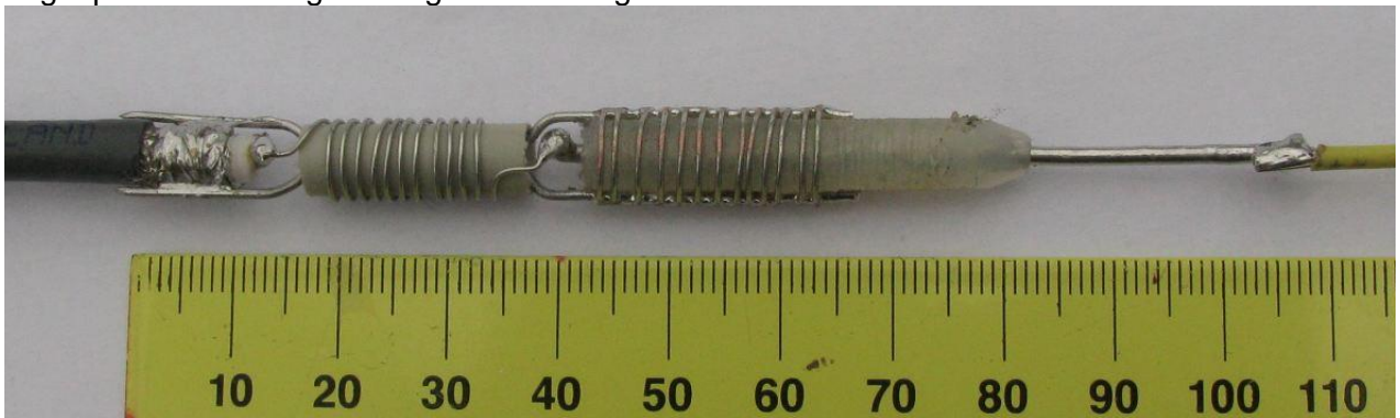
Figure 1.1, light-weight end-fed matching circuit for 2 m band
